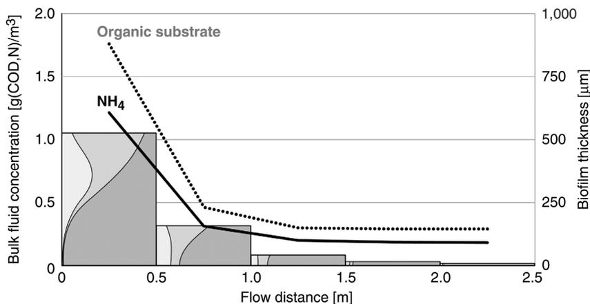
**Figure 9** Pseudo two-dimensional modeling by a series of five biofilm reactor compartments. In the reactor inflow the concentration of organic substrate is 10 gCOD/m<sup>3</sup> and of ammonia 6 gN/m<sup>3</sup>. Inserts show the relative abundance of autotrophic (light gray) and heterotrophic (medium gray) microbial species and of inerts (dark gray) in the biofilm between the substratum (bottom) and the biofilm surface (top)
