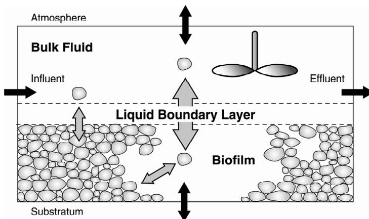
**Figure 1** Setup of the AQUASIM biofilm reactor compartment. Solid arrows indicate possible mass fluxes across compartment boundaries, and shaded arrows indicate mass fluxes within the compartment
