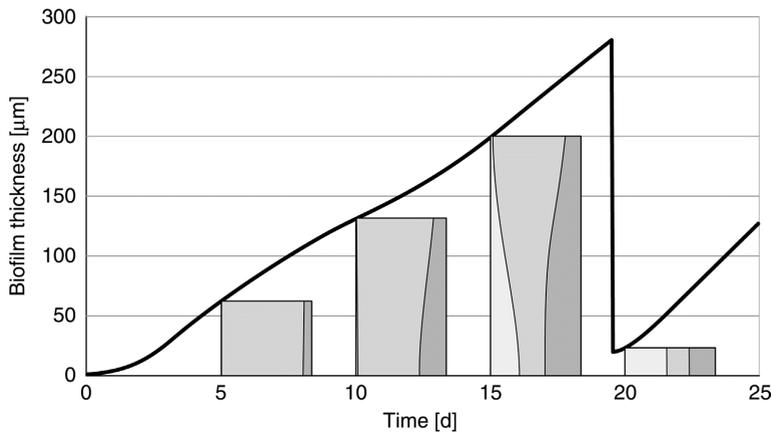
**Figure 7** Biofilm growth and effect of a sloughing event. Inserts show the relative abundance of autotrophic (light gray) and heterotrophic (medium gray) microbial species and of inerts (dark gray) in the biofilm between the substratum (bottom) and the biofilm surface (top)
