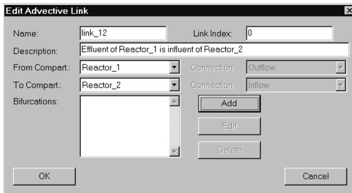
**Figure 8** The AQUASIM dialog box "Edit Advective Link" is used to model water flow and advective substance transport from one compartment to another
