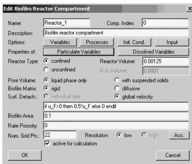
**Figure 2** The AQUASIM dialog box “Edit Biofilm Reactor Compartment” is used to specify the properties of the biofilm system
