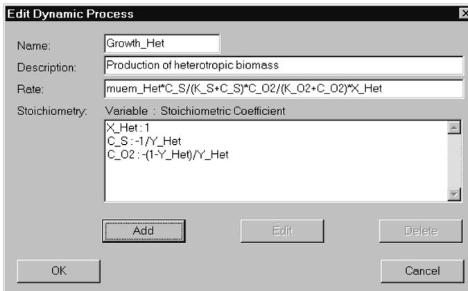
**Figure 3** The AQUASIM dialog box “Edit Dynamic Process” is used to specify the rate laws and stoichiometric coefficients of biotic and abiotic conversion processes
