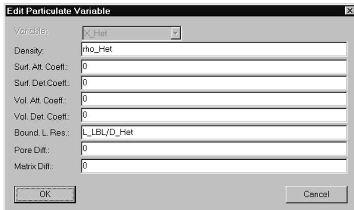
**Figure 4** The AQUASIM dialog box “Edit Particulate Variable” is used to specify the properties of microbial species
