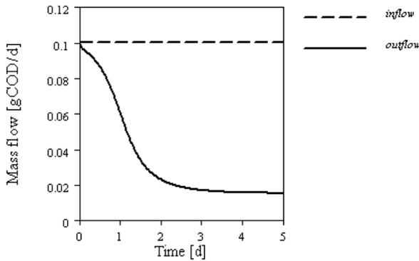
**Figure 6** Typical AQUASIM plot showing the development in time of the reactor inflow and outflow of organic substrate
