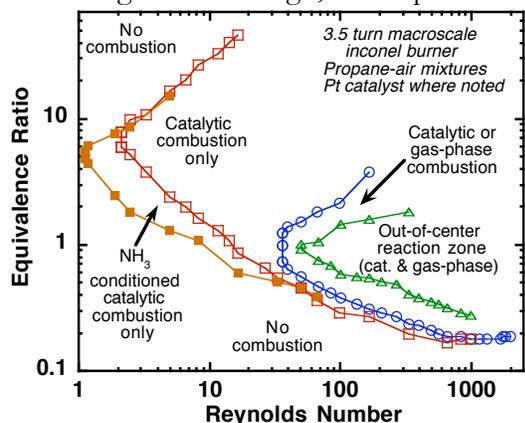
Figure 1. Extinction limits of propane-air mixtures in a 7 cm x 7 cm x 5 cm Swiss roll burner. The case mentioned in the text corresponds to Re = 2184.
