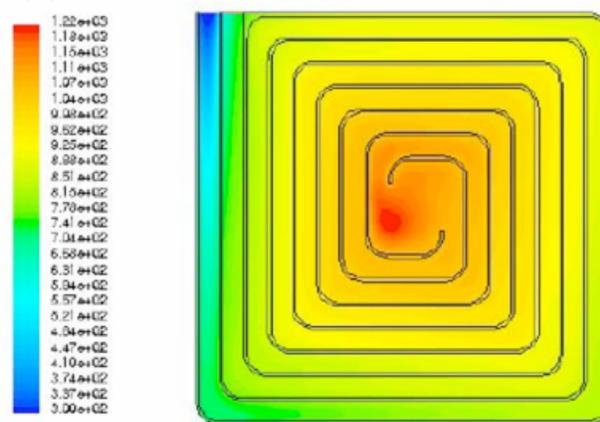
Figure 2. Example of computed temperatures in a Swiss roll combustor including conductive, convective and radiative heat transfer and chemical reaction.
