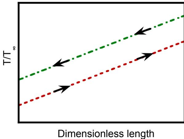
(e) The dividing wall is non-conducting
