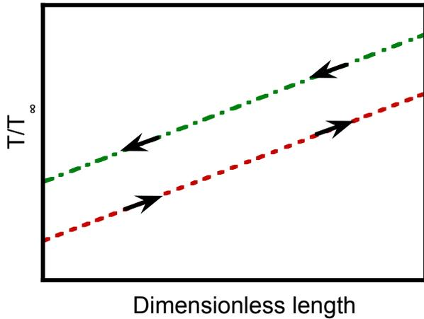
(c) Significant heat losses on reactant side only
