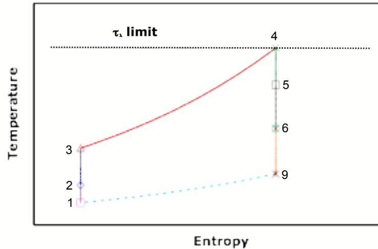
The fan is removed and an afterburner with the same  $\tau_t$  limit as the turbine is added.
