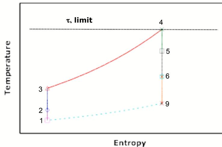
Half way through the standard (constant pressure) burn, abnormal combustion occurs which results in constant **volume** combustion. The same total amount of fuel is burned as in the baseline cycle ( $\tau_t$  limit cannot be honored in this case). All other components operate normally.
